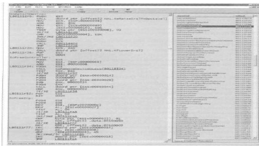
FIGURE 1-8. MFVDasm Disassembling ntoskrnl.exe to DetachDevice()
